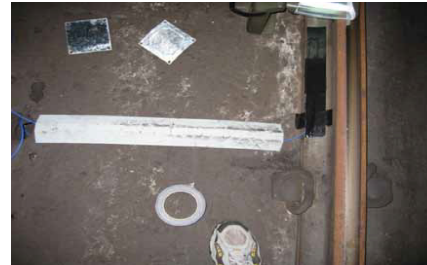
Fig.5. FBG sensor installed on the track
