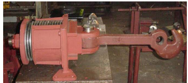
Fig. 1. The buffer assembly filled with the rubber-metal spring
