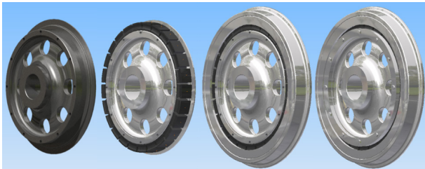
Fig.3. Components of the elastic tram wheel
