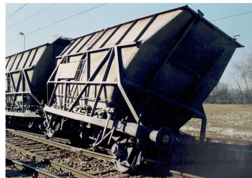
Fig. 1. The derailment of Fbd wagon for coal transportation in thermal power plant “Nikola Tesla” Obrenovac, Serbia
