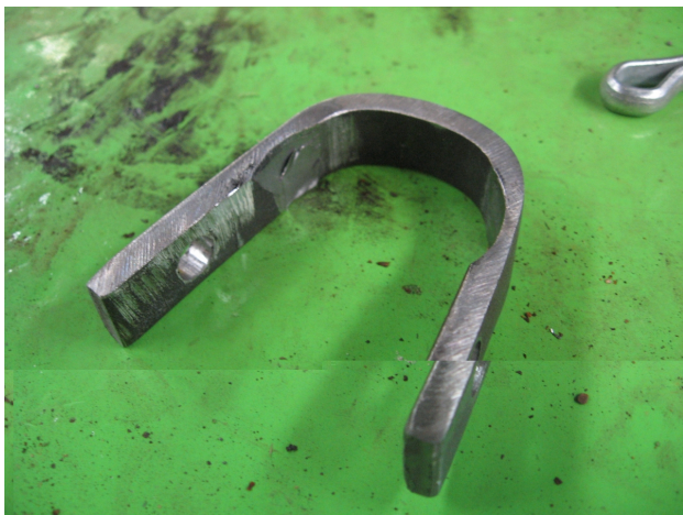
Fig.3. Deformed U-shaped securing element
