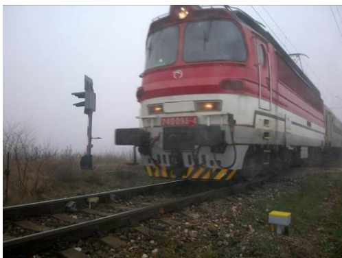
Fig.2. Outdoor devices of BO23 (wheel sensor and trackside box) for train detection on level crossing
