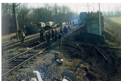
Fig.1. Derailment caused by the axle-bearing failure
