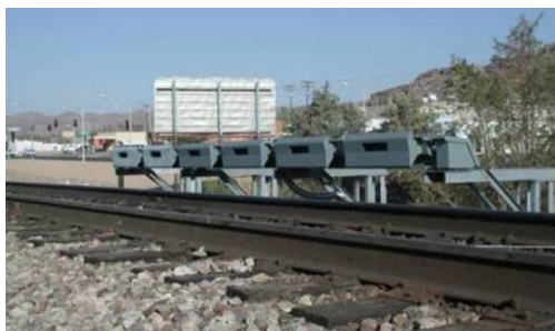
Fig.5. System for acoustic detection of defected bearings on measuring coaches
