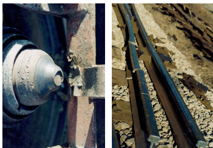
Fig.2. Typical damage of the axle and track
