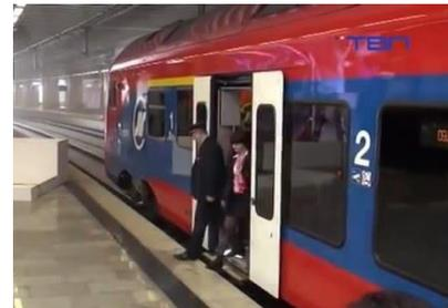
Fig.5. Comfortable and safe access to the platform (platform height 550 mm) from the vehicle
