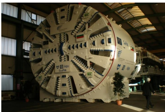
Fig.9. One of Tunnel-boring machine (TBM)
