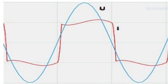
Fig. 2. Current waveform (red) in the AC terminal of the diode rectifier
