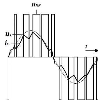
Fig. 6. Current waveform from the AC power network, obtained by PWM in four-quadrant converter
