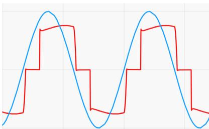
Fig. 4. Current waveform (red) on the AC side of the asymmetric thyristor bridge
