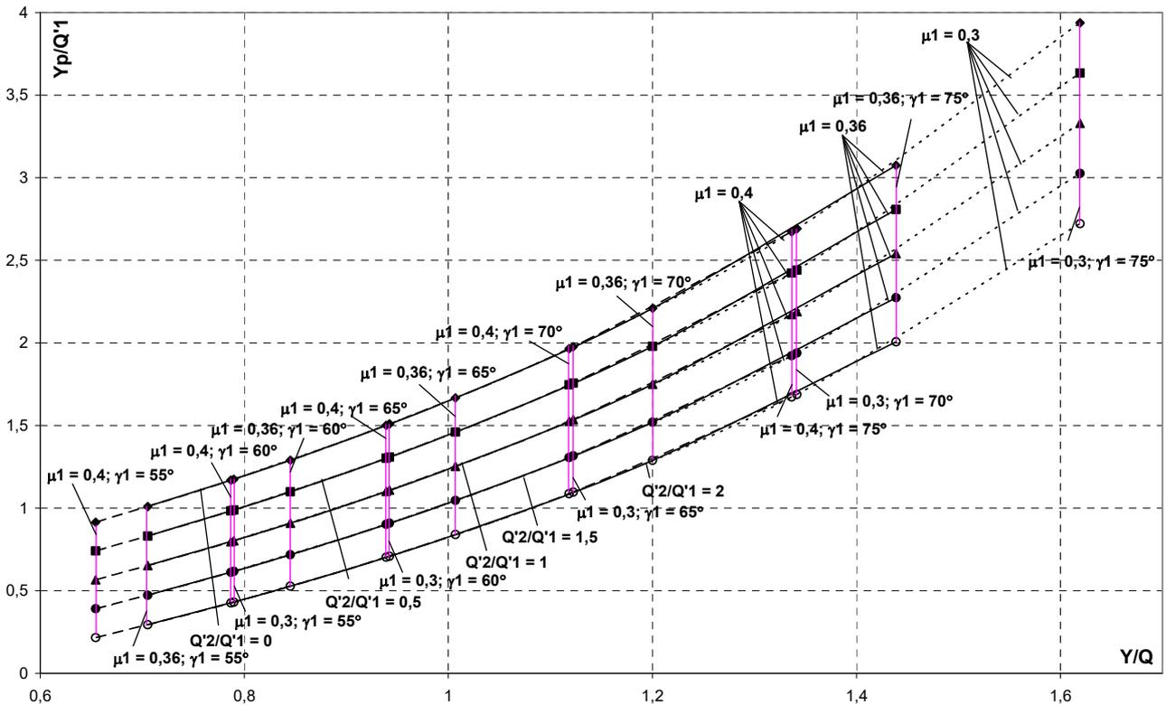
Fig.2 Diagram of  $Y_p/Q'_1$  - nominal criterion against derailment depending on the approved criterion  $Y/Q$  according to EN and UIC, at different values of the parameters  $Q'_2/Q'_1$ ,  $\mu_1$  and  $\gamma_1$ .
