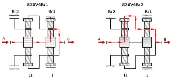
Fig. 5. Power flow through the transmission when the brake Br1 is activated (a) and when the brake Br2 is activated (b)
