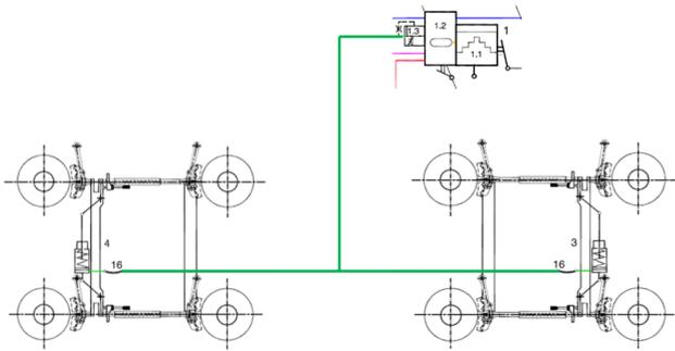
Fig.3. Schematic view of integrated bogie brake system
