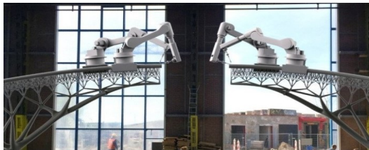
Fig.5. A 3D-printed steel bridge [10]
