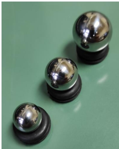
Fig.2. Ball Bearing Samples: 6306, 6308, and 6310 Types
