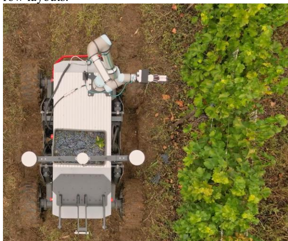
Fig. 11. AgAR platform equipped with a robotic system for grape harvesting
