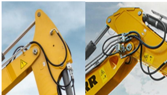
Fig 1. Left - previous solution of the connection of the first and second hand, right - the new solution [3]
