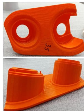
Fig.8. Fixture for positioning headlights for the front fairing of the train
