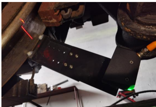
Fig. 2. Wheel rim profile scanning [13]
