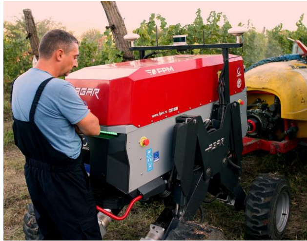
Fig.8. Emergency stop when bumper is activated
