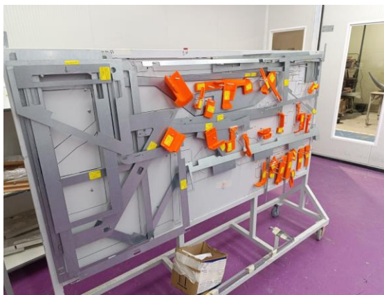
Fig.9. Sheet metal and additively manufactured fixtures
