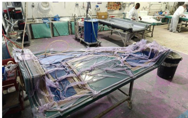
Fig.2. Appearance of the composite after the infusion process
