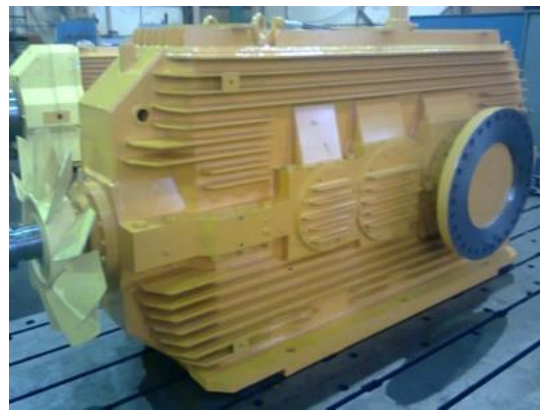
Fig.4. Gearboxes with fan on proof-stand
