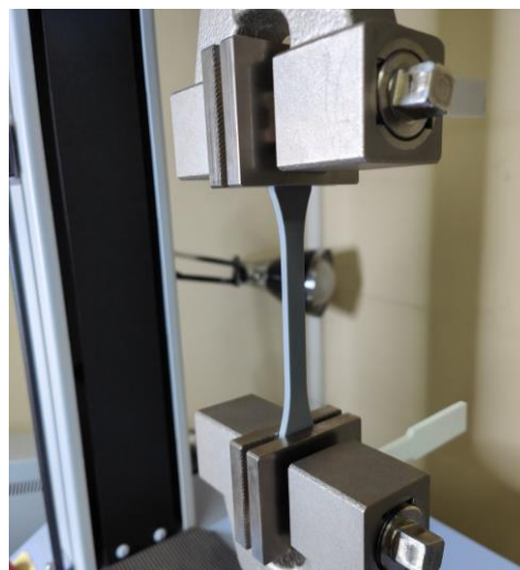
Fig.3. Shimadzu AGS-X Universal Testing Machine with a specimen
