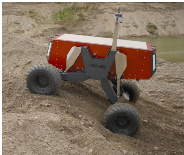
Fig.9. AgAR on a 40° slope with levelling system activated
