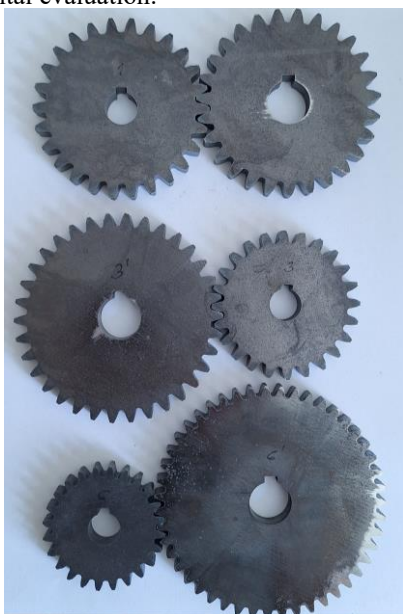
Fig. 2. Laser-cut produced spur gear pairs
