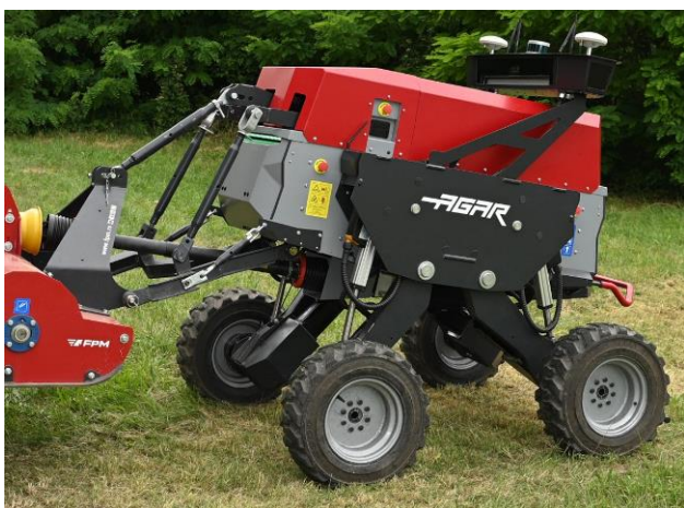
Fig.8. AgAR 3-point hitch subsystem and a sensor bridge
