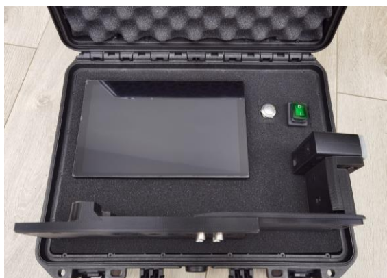
Fig. 4. Laser measuring device housed in its portable suitcase for wheel rim inspection [13]
