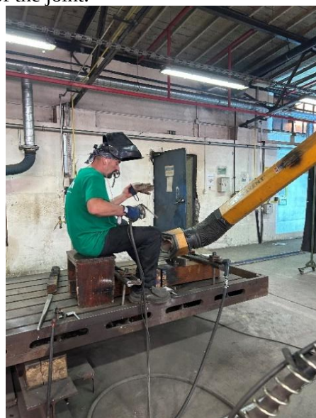
Fig 5. SS-FCAW welding process
