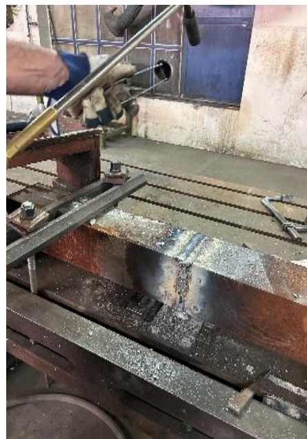
Fig 7. SS-FCAW welded specimen
