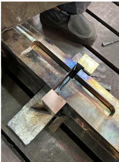
Fig 6. Appearance of the welded joint prior to hardfacing
