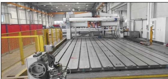
Fig. 1. FSW welding machine
