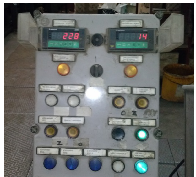
Fig. 9. Indicating gauge on the control panel device for tensioning wire
