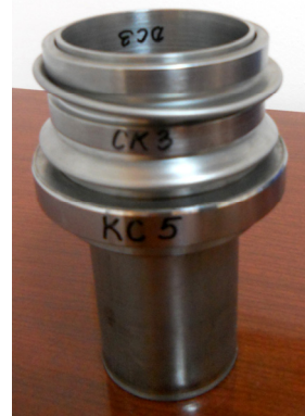
Fig. 6. Deformed shrinking-folding absorber
