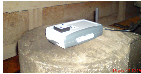
Picture 2. Accelerometer placed on the cup of the spring from the ASR..
