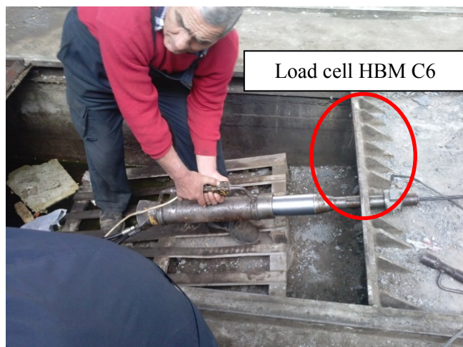
Fig. 2. Measurement of force in the prestressing cables
