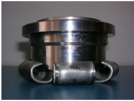
Fig. 8. Deformed shrinking-splitting absorber
