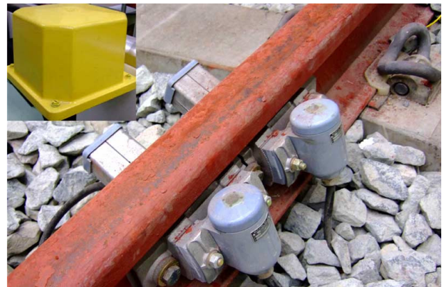
Fig.1. Axle counter consists of two pairs of transmitter and receiver [2]
