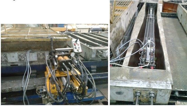
Fig. 5. System for tensioning the wire in the tool for concrete sleepers used from DIV Svrlijig
