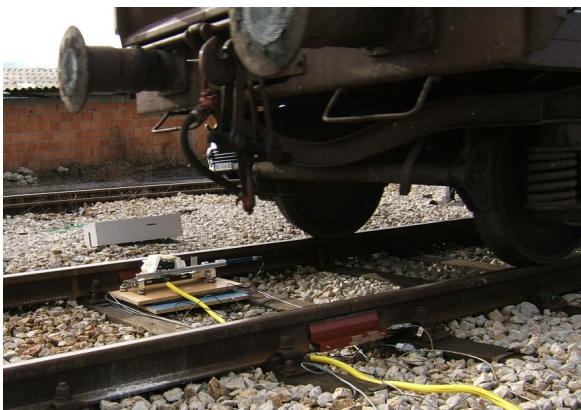
Fig. 2. Trailing unit EMU 416-077 – angle of attack measurement device without protective cover
