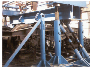
Fig. 4. General type of a device for testing dynamic fatigue of freight bogies.
