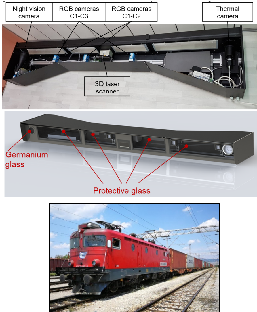
Fig. 2 (top) Final sensors' housing of the integrated SMART ODS demonstrator with the integrated sensors labelled. (middle) CAD model of the closed sensors' housing with protective glass labelled. (bottom) Frontal profile of a SMART test vehicle, Serbia Cargo ŽS series 441, with the ODS demonstrator mounted under the headlights
