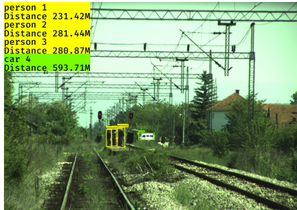
Fig. 12. Mid- to Long-range object detection and distance estimation in on-board RGB camera image; Ground truth distance: for persons (station middle point) 266,69 m (average error 8,32%), for the car 597,87 m (error 0,69%)
