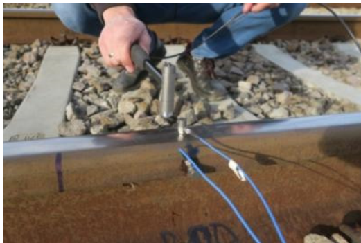
Fig. 4. Instrumented hammer impact for direct FRF
