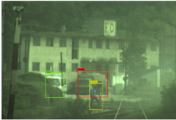
Fig. 7. Real-world scene: (left) person crossing the rail tracks on unsecured crossing “Momin Kamen” while train is approaching. Vehicles parked near the rail tracks; (right) vehicle suddenly changed the status from “parked” to “moving vehicle crossing the rail tracks on unsecured crossing “Momin Kamen” while train is approaching
