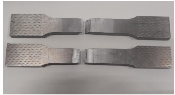
Fig. 9. Specimen failure site
