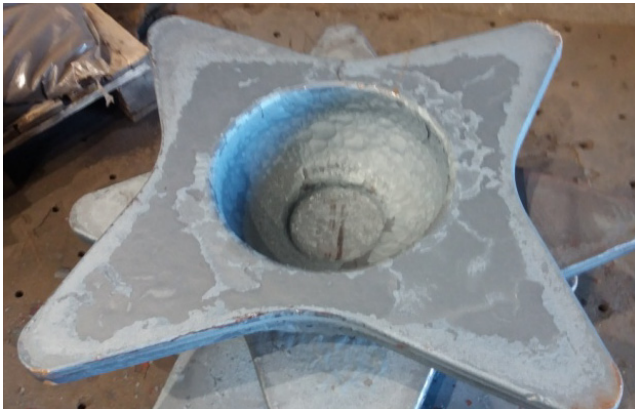
Fig. 5. Finished part with directions of geometric inaccuracies of forging in radial flow
