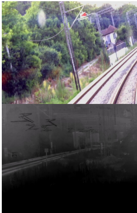
Fig.13. Rail tracks curve as seen from the fixed view on-board RGB camera (top), controlled view on-board thermal camera (bottom)
