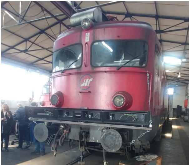
Fig.5. Trial mounting of the ODS demonstrator onto the locomotive series 444 in the in Niš locomotive depot workshop
