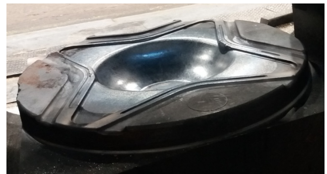
Fig.4. Filling the warehouse of surplus material in the final shape of forging
