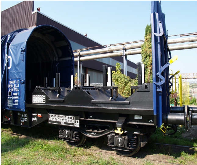
Fig.1. Partially uncovered Shimmns wagon
