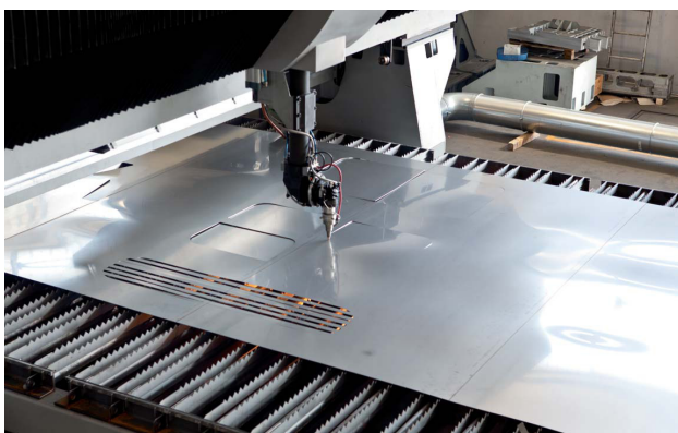
Fig.3. 2D Laser cutting on the openings in a railway vehicle's side wall [8]
