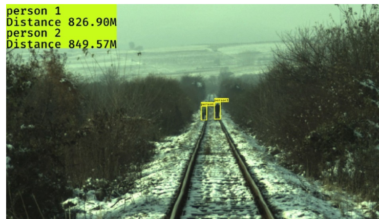
Fig. 10. Object detection and distance estimation in RGB camera image recorded in winter (snow) environmental conditions; Ground truth distance: 835 m (error 0,97 % and 1,74% respectively)
