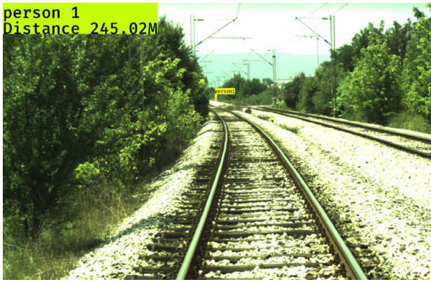
Fig. 11. (left) Mid-range object detection and distance estimation in on-board RGB camera image; Ground truth distance: 272,75 m (error 10%); (right) Mid-range object detection and distance estimation in on-board RGB camera image; Ground truth distance: 231,97 m (errors 8,2% and 8,24% respectively)
