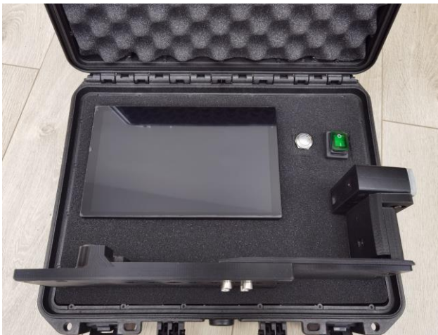
Fig. 7. Laser measuring device housed in its portable suitcase for wheel rim inspection
