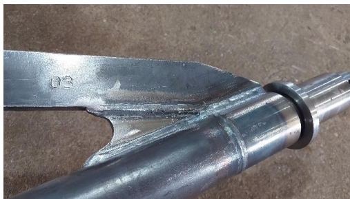
Fig.3. Welded brake triangle
