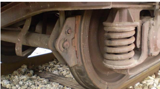
Fig.1. Braking elements of freight wagon
