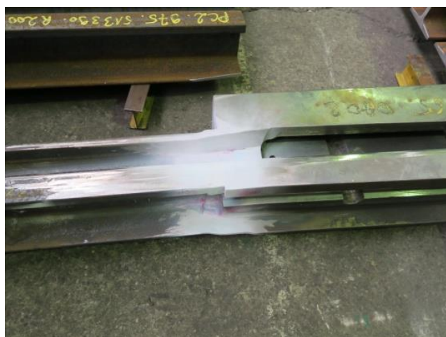
Fig. 4. Welded rail-block joint
