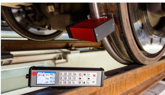
Fig. 1. Device for measuring wheel rim parameters [4]
