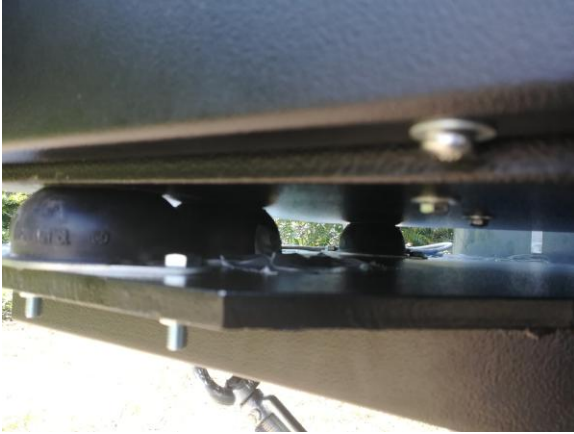
Fig. 2. Viscoelastic elements for vibration suppression
