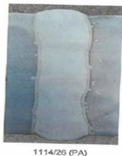
Fig 10. Macrosection of the specimen welded using the SS-FCAW process
