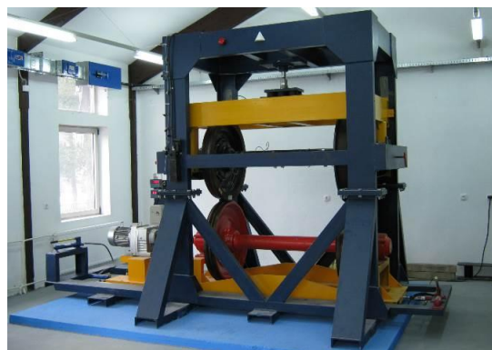
Fig.1. Test stand for testing and calibration of measuring wheelsets [4, 5]
