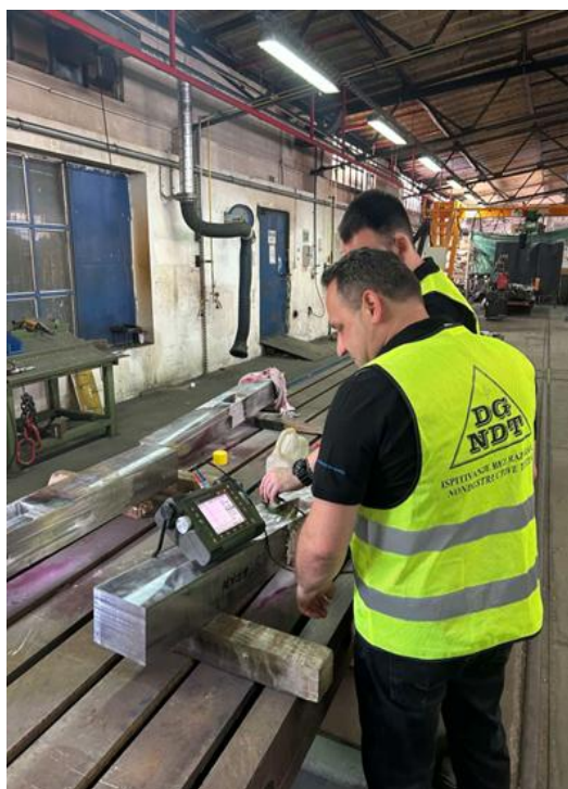
Fig 8. Ultrasonic testing of the welded joint
