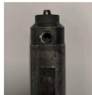
Fig. 2. FSW tool geometry
