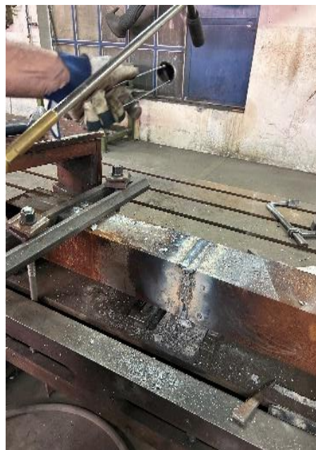
Fig 7. SS-FCAW welded specimen
