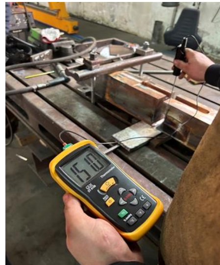
Fig 3. Preheating temperature control
